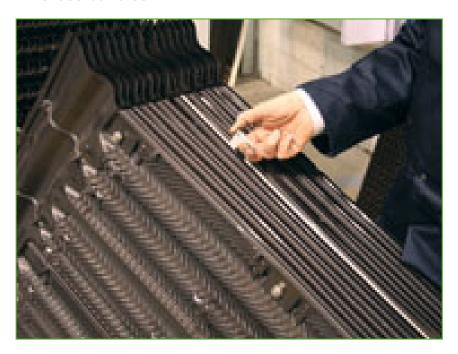
BACross bundles include <u>BACross fill sheet packs</u> with an handle to hang the bundles on the fill support.
