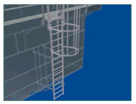
A ladder, safety cage and handrails are all installed for **easy access to the unit top and easier and safer** inspection and maintenance, in line with **EU safety directives**. For units equipped with these options, we also recommended installing steel drift eliminators.
