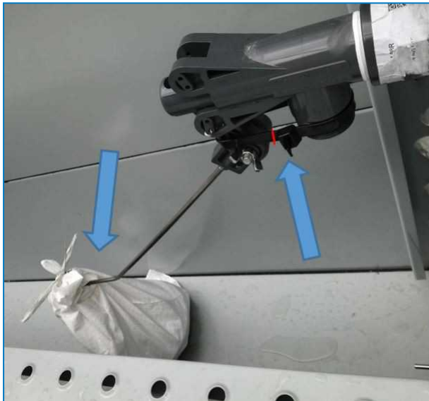
Fixation and wrapping of float ball
