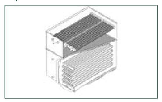
Ammonia (R-717) reciprocating compressors give off highly superheated gas, which should be **cooled** via the desuperheater coil before it enters the condensing coil.
